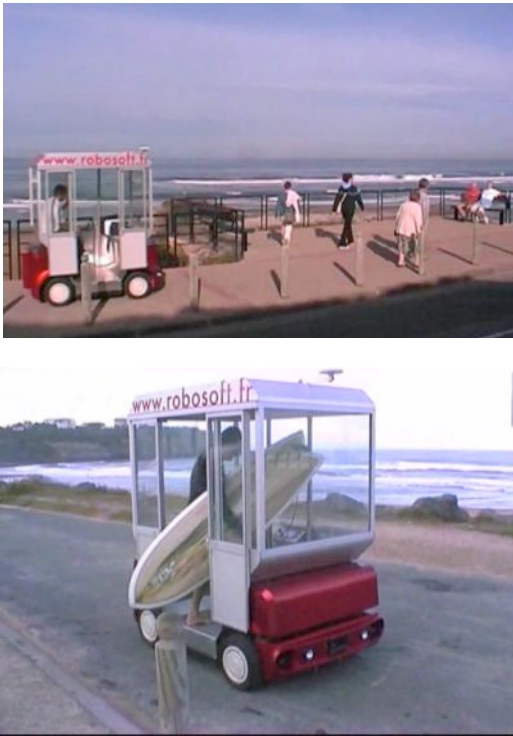
Fig. 5: Anglet experiment: using the robuCAB as a CTS in a crowded pedestrian area
