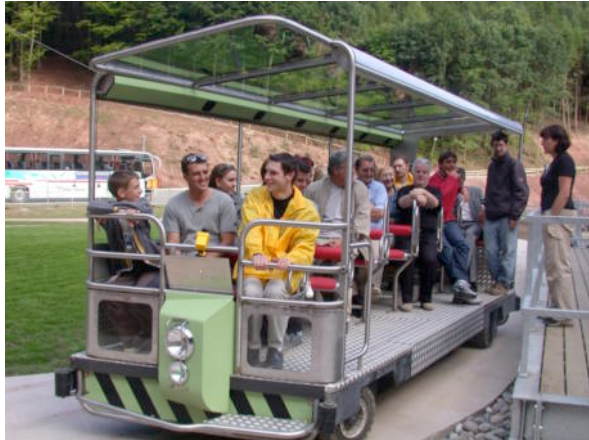
Fig. 3: Simserhof entertainment park. CyberCars using embedded wires.
